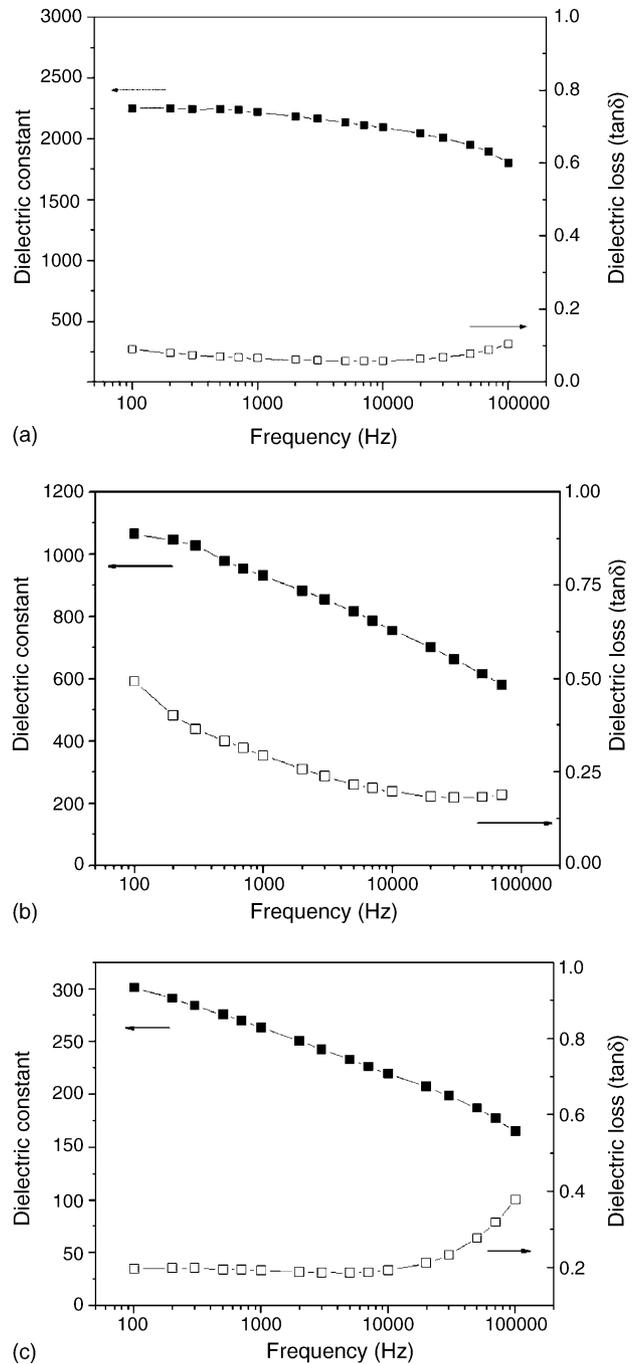
Fig. 3. Frequency dependence of the dielectric constant and dielectric loss of the (a)  $\text{Pb}_{0.8}\text{Ba}_{0.2}\text{TiO}_3$ ; (b)  $\text{Pb}_{0.6}\text{Ca}_{0.4}\text{TiO}_3$ ; and (c)  $\text{PbZr}_{0.3}\text{Ti}_{0.7}\text{O}_3$  thin films.
