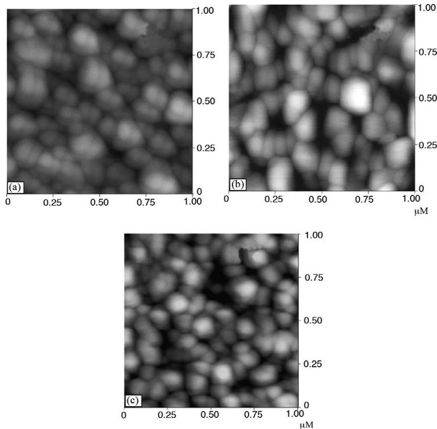
Fig. 2. AFM micrographs of the (a)  $\text{Pb}_{0.8}\text{Ba}_{0.2}\text{TiO}_3$  thin films; (b)  $\text{Pb}_{0.6}\text{Ca}_{0.4}\text{TiO}_3$  thin film; and (c)  $\text{PbZr}_{0.30}\text{Ti}_{0.70}\text{O}_3$  thin film. S represents the substrate peaks.
