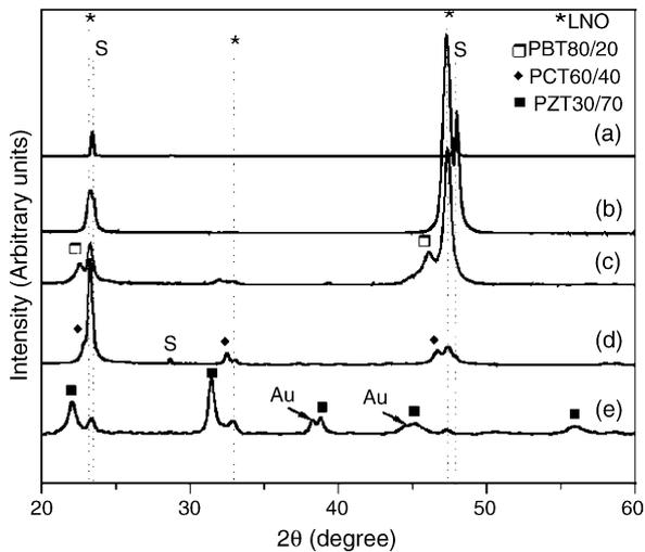
Fig. 1. X-ray patterns of (a)  $\text{LaAlO}_3$  substrate; (b)  $\text{LaNiO}_3$  thin film on the substrate; (c)  $\text{Pb}_{0.8}\text{Ba}_{0.2}\text{TiO}_3$  thin film on  $\text{LaNiO}_3/\text{LaAlO}_3$  (100);  $\text{Pb}_{0.6}\text{Ca}_{0.4}\text{TiO}_3$  thin film on  $\text{LaNiO}_3/\text{LaAlO}_3$  (100); and (e)  $\text{PbZr}_{0.30}\text{Ti}_{0.70}\text{O}_3$  thin film on  $\text{LaNiO}_3/\text{LaAlO}_3$  (100). S, substrate peak.
